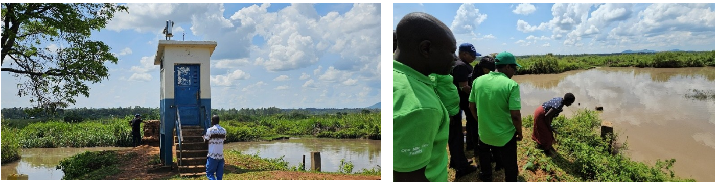
Figure 14: Automated gauge station (Left); Mrs. Alice Okech reading the water levels (Right) in Bunadeti-Nahusi
